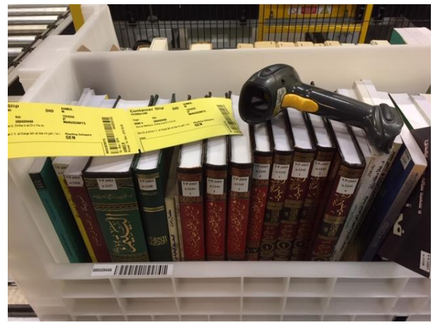
Tote bar code linked to each item. Operator selects item and bar code wands – item and ticket.
